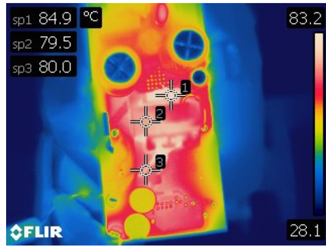
Figure 17 – Top Side. 85 VAC, Full Load. Sp1 – Transformer Secondary Winding – 84.9 °C. Sp2 – Transformer Core – 79.5 °C. Sp3 – Transformer Wire Secondary Winding – 80 °C.
