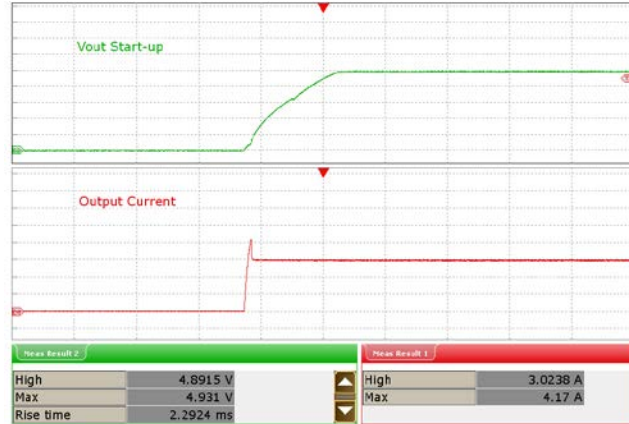
Figure 21 – V_{IN} = 85 \text{ VAC} , Full Load. C2 Green: V_{OUT} , 1 V / div., 2 ms / div. C4 Red: I_{OUT} , 1 A / div., 2 ms / div. V_{OUT(MAX)} = 4.93 \text{ V} .
