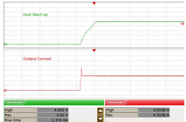
Figure 27 – V_{IN} = 265 VAC, Full Load. C2 Green: V_{OUT} , 1 V / div., 2 ms / div. C4 Red: I_{OUT} , 1 A / div., 2 ms / div. V_{OUT(MAX)} = 5.01 V.
