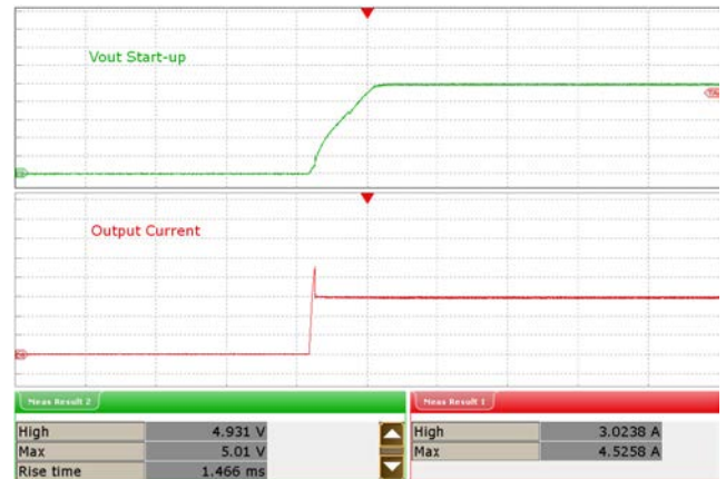
Figure 25 – V_{IN} = 230 VAC, Full Load. C2 Green: V_{OUT} , 1 V / div., 2 ms / div. C4 Red: I_{OUT} , 1 A / div., 2 ms / div. V_{OUT(MAX)} = 5.01 V
