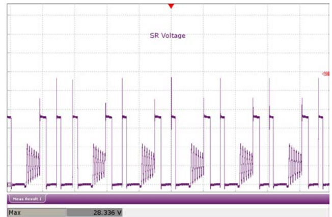
Figure 41 – V_{IN} = 115 \text{ VAC} . C2 Violet: V_{SRFET} , 5 V / div., 20 \mu\text{s} / div. V_{DS(MAX)} = 28 \text{ V} .
