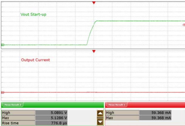
Figure 24 – V_{IN} = 230 VAC, No Load. C2 Green: V_{OUT} , 1 V / div., 2 ms / div. C4 Red: I_{OUT} , 1 A / div., 2 ms / div. V_{OUT(MAX)} = 5.12 V
