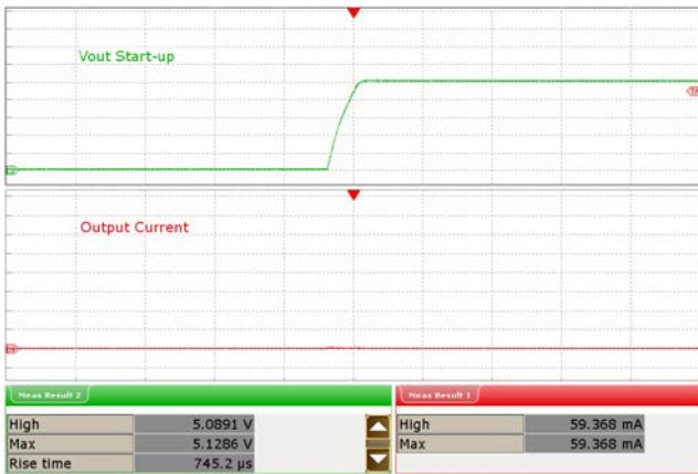
Figure 26 – V_{IN} = 265 VAC, No-Load. C2 Green: V_{OUT} , 1 V / div., 2 ms / div. C4 Red: I_{OUT} , 1 A / div., 2 ms / div. V_{OUT(MAX)} = 5.12 V.
