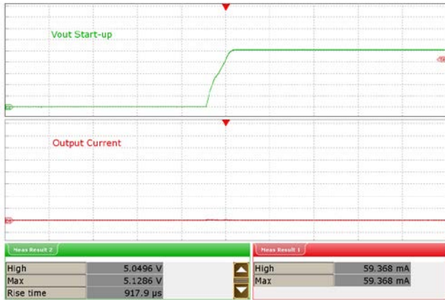
Figure 20 – V_{IN} = 85 \text{ VAC} , No-Load. C2 Green: V_{OUT} , 1 V / div., 2 ms / div. C4 Red: I_{OUT} , 1 A / div., 2 ms / div. V_{OUT(MAX)} = 5.12 \text{ V} .
