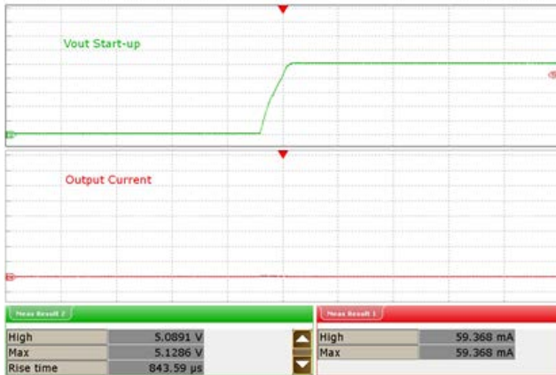
Figure 22 – V_{IN} = 115 \text{ VAC} , No-Load. C2 Green: V_{OUT} , 1 V / div., 2 ms / div. C4 Red: I_{OUT} , 1 A / div., 2 ms / div. V_{OUT(MAX)} = 5.12 \text{ V} .
