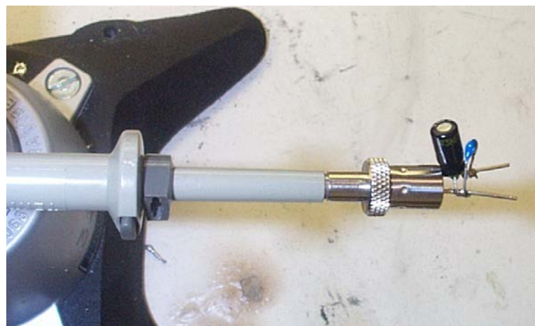
Figure 79 – Oscilloscope Probe with Probe Master ( www.probemaster.com ) 4987A BNC Adapter. (Modified with wires for ripple measurement, and two parallel decoupling capacitors added.)
