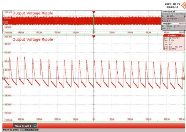
Figure 86 – 230 VAC 50 Hz. CH1: V_{OUT} , 20 mV / div., 10 ms / div. Zoom: 50 \mu s / div. Output Ripple = 80.632 mV.
