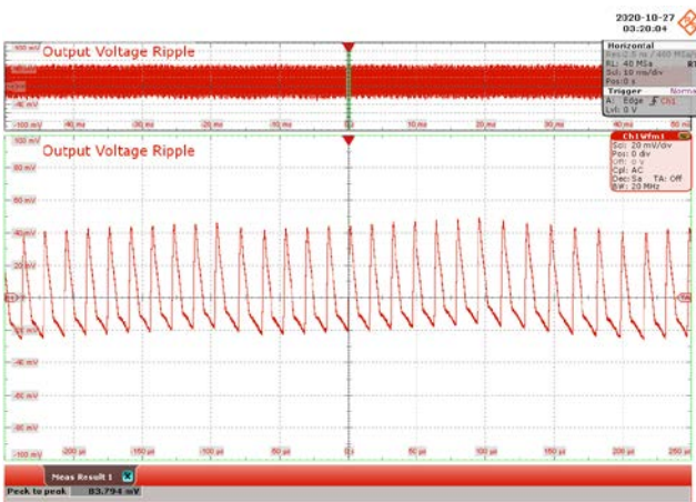
Figure 82 – 230 VAC 50 Hz. CH1: V_{OUT} , 20 mV / div., 10 ms / div. Zoom: 50 \mu s / div. Output Ripple = 83.794 mV.
