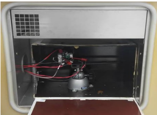
Figure 98 – Thermal Performance Set-up Using Thermal Chamber.
