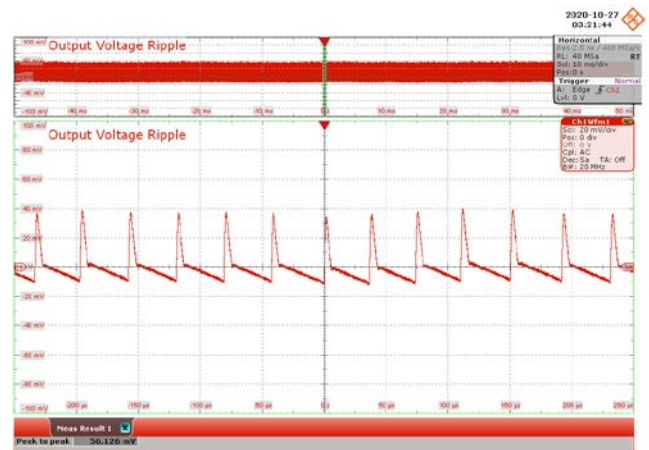
Figure 95 – 265 VAC 50 Hz. CH1: V_{OUT} , 20 mV / div., 10 ms / div. Zoom: 50 \mu s / div. Output Ripple = 56.126 mV.
