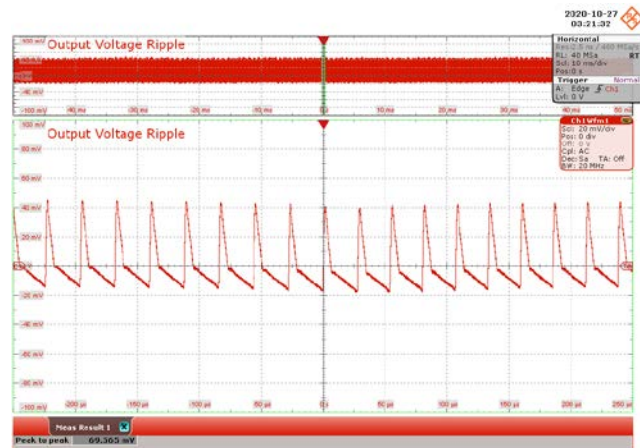
Figure 91 – 265 VAC 50 Hz. CH1: V_{OUT} , 20 mV / div., 10 ms / div. Zoom: 50 \mu s / div. Output Ripple = 69.565 mV.
