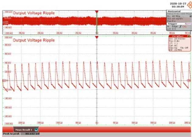
Figure 84 – 90 VAC 60 Hz. CH1: V_{OUT} , 20 mV / div., 10 ms / div. Zoom: 50 \mu s / div. Output Ripple = 80.632 mV.
