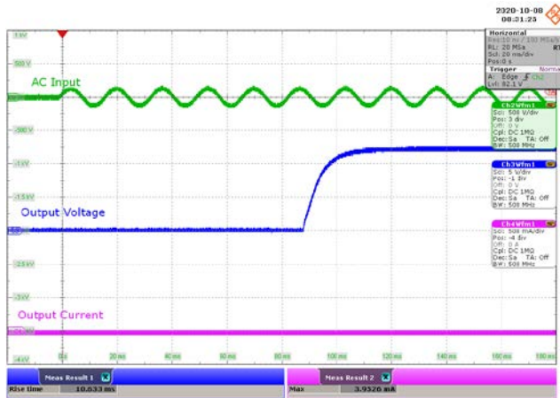
Figure 34 – 85 VAC 60 Hz. CH2: V_{IN} , 500 V / div., 20 ms / div. CH3: V_{OUT} , 5 V / div., 20 ms / div. CH4: I_{OUT} , 500 mA / div., 20 ms / div. Rise Time = 10.633 ms.
