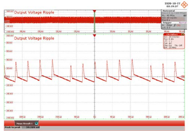
Figure 93 – 115 VAC 60 Hz. CH1: V_{OUT} , 20 mV / div., 10 ms / div. Zoom: 50 \mu s / div. Output Ripple = 59.289 mV.
