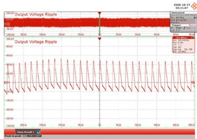
Figure 83 – 265 VAC 50 Hz. CH1: V_{OUT} , 20 mV / div., 10 ms / div. Zoom: 50 \mu s / div. Output Ripple = 84.585 mV.
