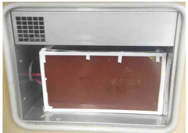
Figure 98 – Thermal Performance Set-up Using Thermal Chamber.
