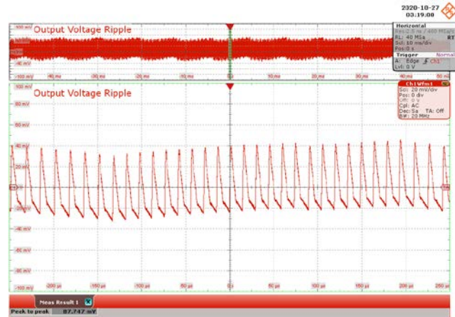
Figure 81 – 115 VAC 60 Hz. CH1: V_{OUT} , 20 mV / div., 10 ms / div. Zoom: 50 \mu s / div. Output Ripple = 87.747 mV.
