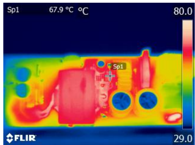
Figure 54 – R1 – Line Voltage Sense Resistor. Spot: 67.9 °C.
