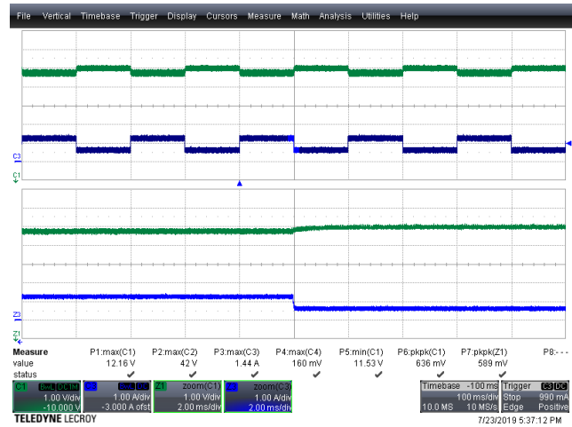
Figure 94 – Output Load Transient, 100% to 50% Load. V_{IN} = 60 \text{ VDC} , I_{OUT} = 1.25 \text{ A} to 0.625 \text{ A} . V_{OUT(MAX)} = 12.16 \text{ V} , V_{OUT(MIN)} = 11.53 \text{ V} . Upper: V_{OUT} , 1 V, 100 ms / div. Lower: I_{OUT} , 1 A, 100 ms / div. Bottom Half: Zoom @ 2 ms / div.
