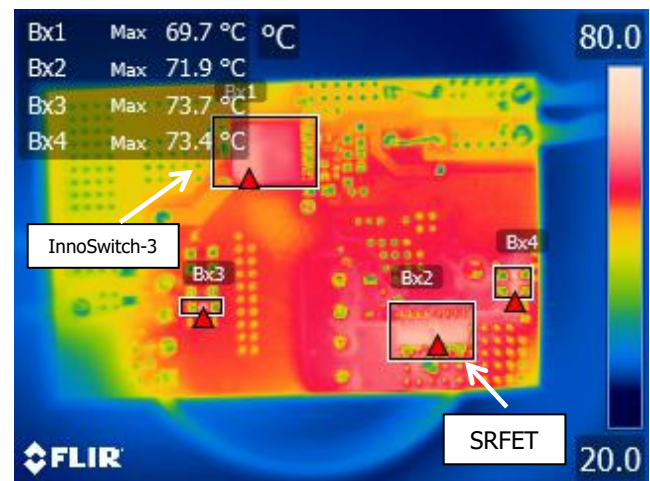
Figure 109 – 400 VDC 2.5 A Full Load. Temperature of InnoSwitch3-AQ: 69.7 °C. Temperature of SR FET: 71.9 °C. Ambient Temperature: 26.8 °C.
