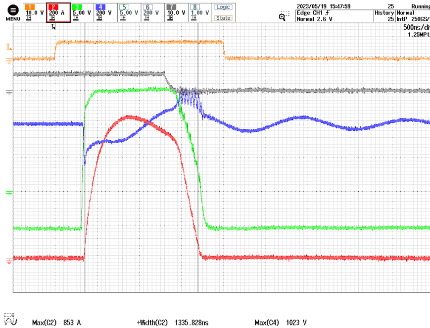
Figure 87 – Top Channel Short Circuit Response at T_j = 25^\circ\text{C} , measured t_{sc} = 1.335 \mu\text{s}
