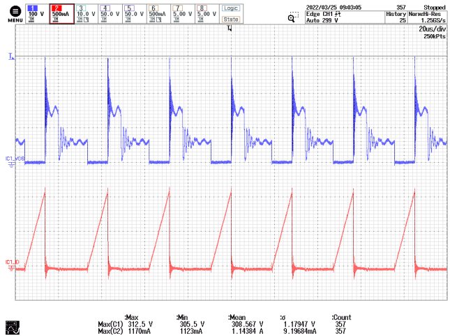
Figure 47 – INN3947CQ Drain Voltage and Current. 60 V DC , 1.333 A Load. CH1: V DS , 100 V / div. CH2: I D , 500 mA / div. Time: 10 µs / div.
