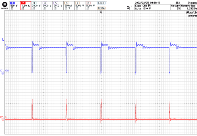
Figure 48 – INN3947CQ Drain Voltage and Current. 800 V DC , 1.333 A Load. CH1: V DS , 500 V / div. CH2: I D , 1 A / div. Time: 20 μs / div.
